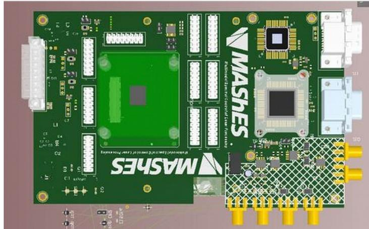
Figure 2 MASHES multisensor board
